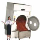
Forward tilt drops the load into a trolley within 30 sec. **Savings on time & labor.**
